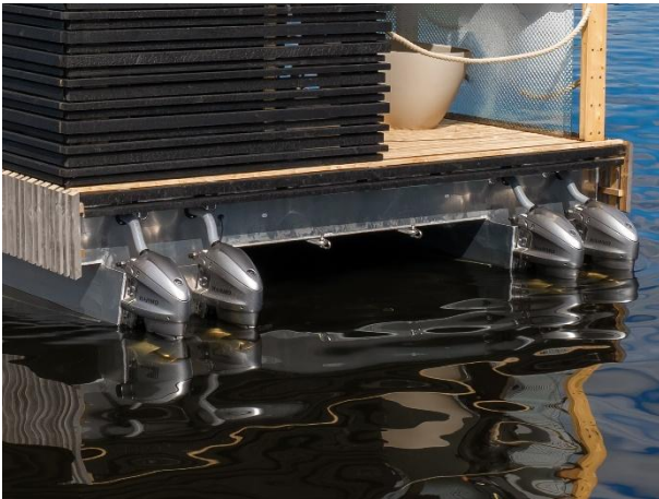
Yamaha Motor's HARMO electric propulsion system on the hydrogen-powered sauna boat.
